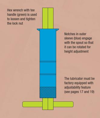
Fig. 10 - Adjusting the Spout Height on B2305 and B2311
