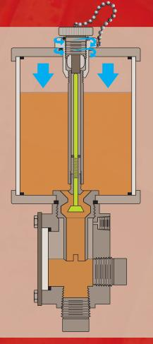
A partially open cap allows air (blue) to flow past the threads
