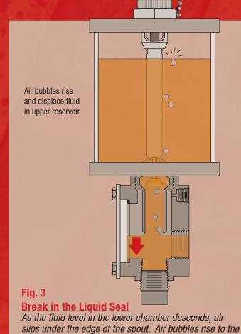
upper reservoir where they displace fluid. The displaced
