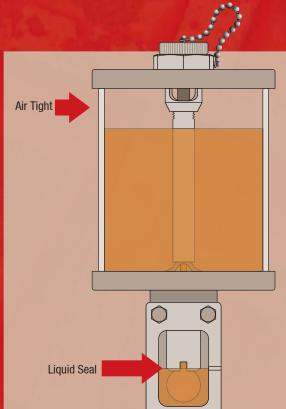
Fig. 2 Upper Reservoir Seal
