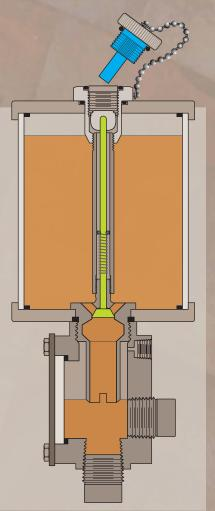
Fig. 12 - Oil Retention **During Reservoir Refills**
